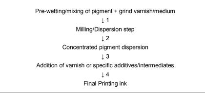
In manufacturing of some inks (notably whites) the intermediate concentrate production (Step 2) can be avoided through adding all necessary additives prior to milling step 1, thus producing a finished ink in a single step.
